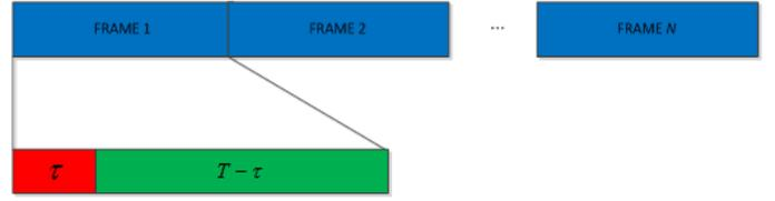
Fig.1. listen-before-transmit frame structure for cognitive radio networks
